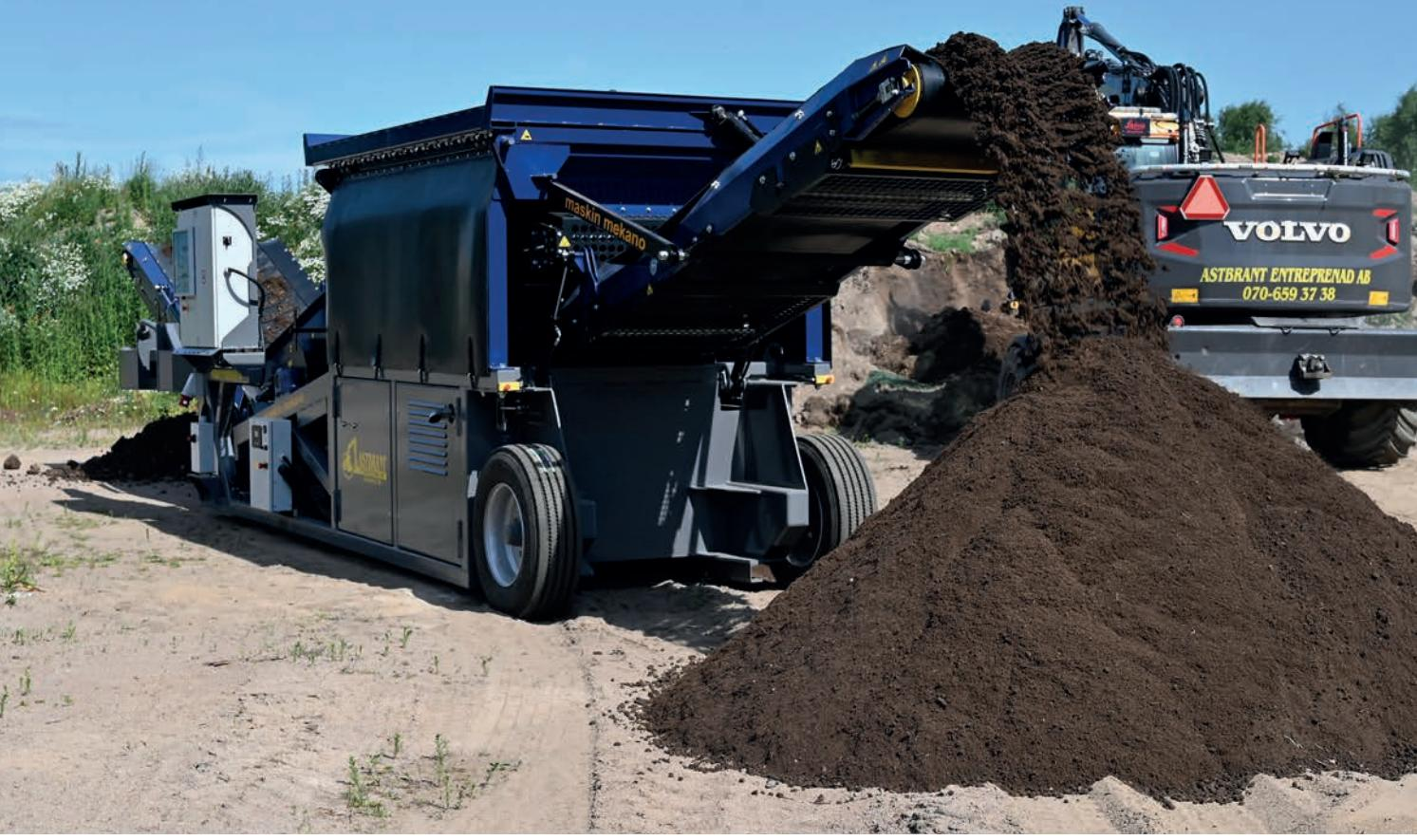
efficient. The Vibroblock design allows the STE screen to operate with the capacity of a four bearing screen, smoother than a two bearing screen, and keeps the power in the screen-box where it belongs.
