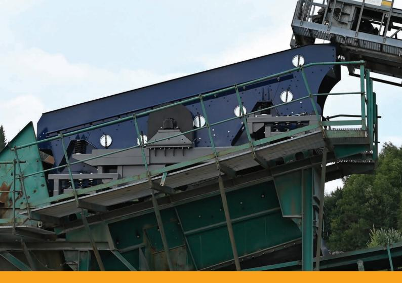
Thanks to the innovative Vibroblock concept, both the screen and motor are mounted on a fully vibration-isolated frame. This allows us to use a high-stroke STE screen for maximum screening efficiency—without any vibrations transferring to the chassis. The result? Superior performance with zero risk of vibration-related wear or damage to the rest of the machine.
